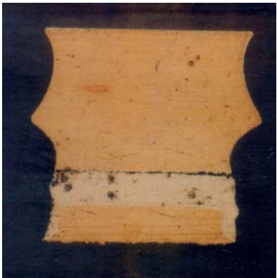
Figure 10: Failed Solder Joint. SnPb lead finish, SnAgCu Solder Paste, OSP board. This is a Corner Pin Located Adjacent to that shown in Figure 9.
