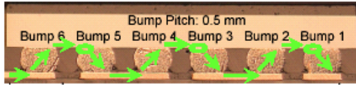
Figure 1. Cross-sectional SEM image. Electron flow (green) for one side of test die.
