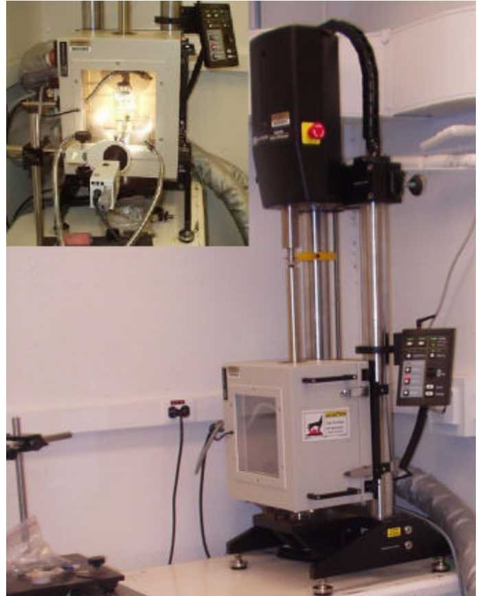
Fig 5: Experimental setup combined with the DIC characterization with tensile testing using Instron 5848 Micro Tester
