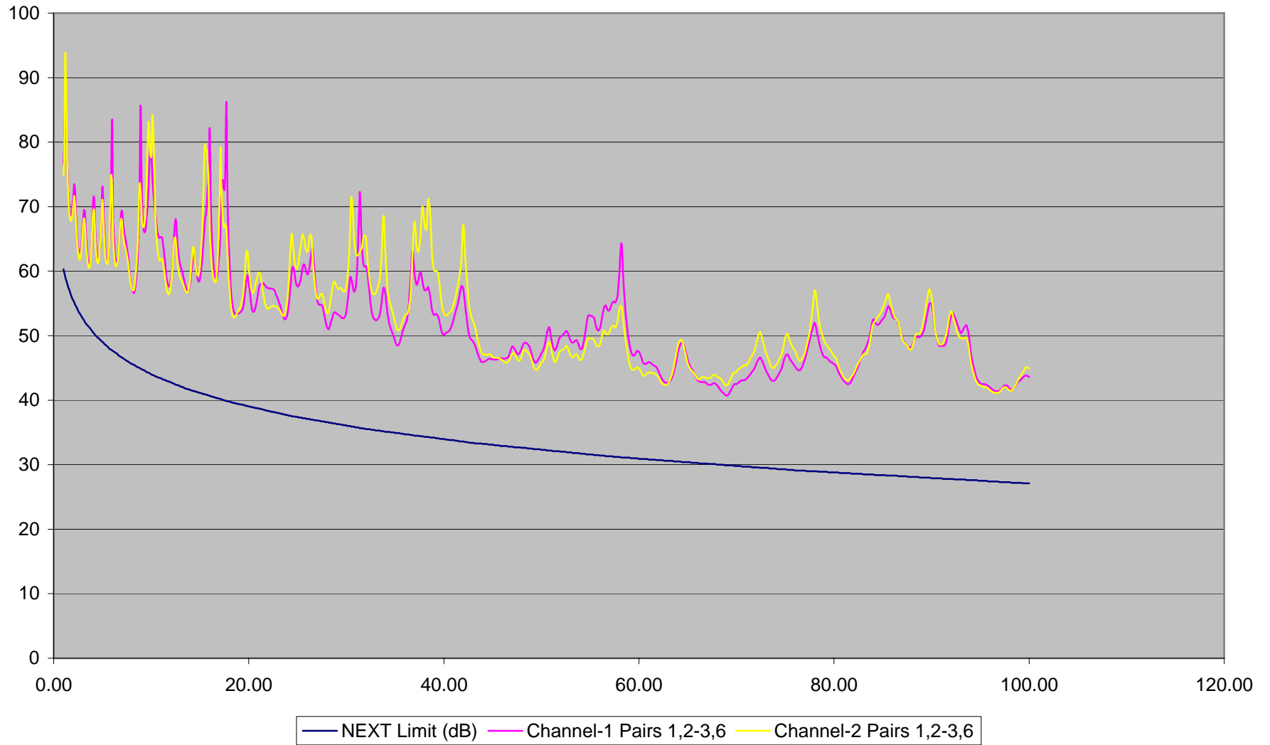
CAT 5 - TSB95 Spec @ Maximum Attenuation - Near End Cross Talk X-Axis Frequency (MHz), Y-Axis NEXT (dB)
