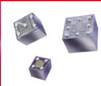
Footprint to Die Ratios of Standard Surface Mount Packages vs. Micro SMD
