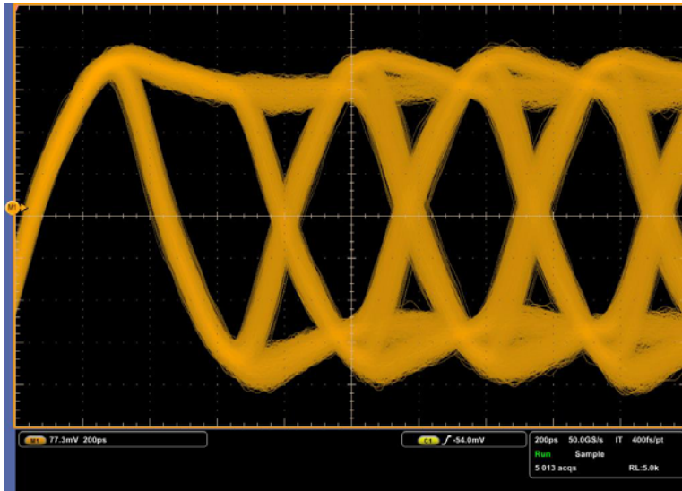
Figure 3. Eye Pattern at 2.7 Gbps / 2 meters / TP0
