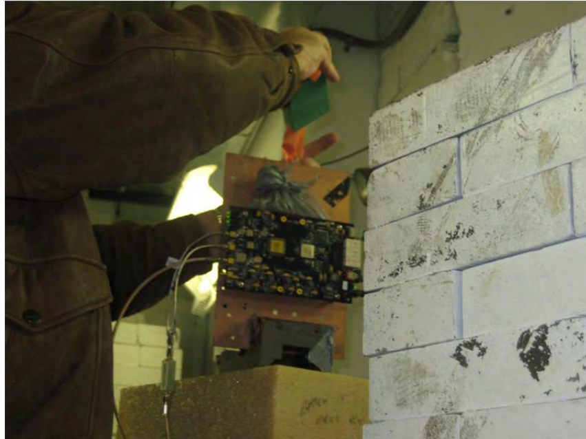
Fig. 11: Test board attached to holding plate, with bag of shredded borated polyethylene between the board and plate to shield from secondary neutrons.
