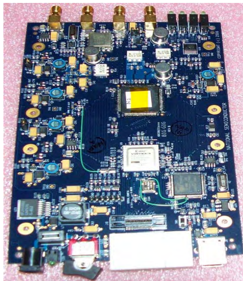
Fig. 2: ADC08D1000DEV board with decapped DUT.
