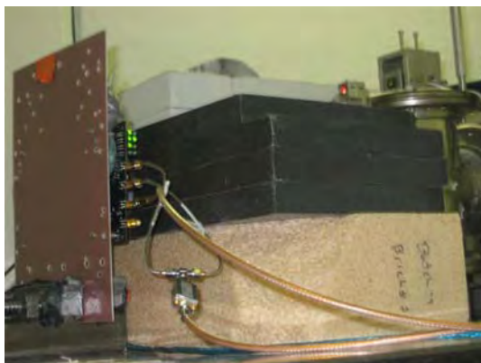
Fig. 12: Backside of board with beam line shielding.
