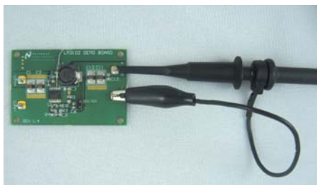
Figure 8. Poor Measurement Technique
