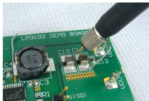
Figure 7. Good Measurement Technique to Measure Output Ripple Voltage
