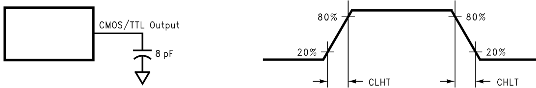
FIGURE 4. DS90CF386 (Receiver) CMOS/TTL Output Load and Transition Times
